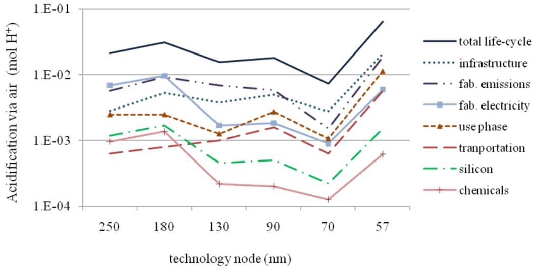
Figure 6.5. Acidification per OS by technology node
