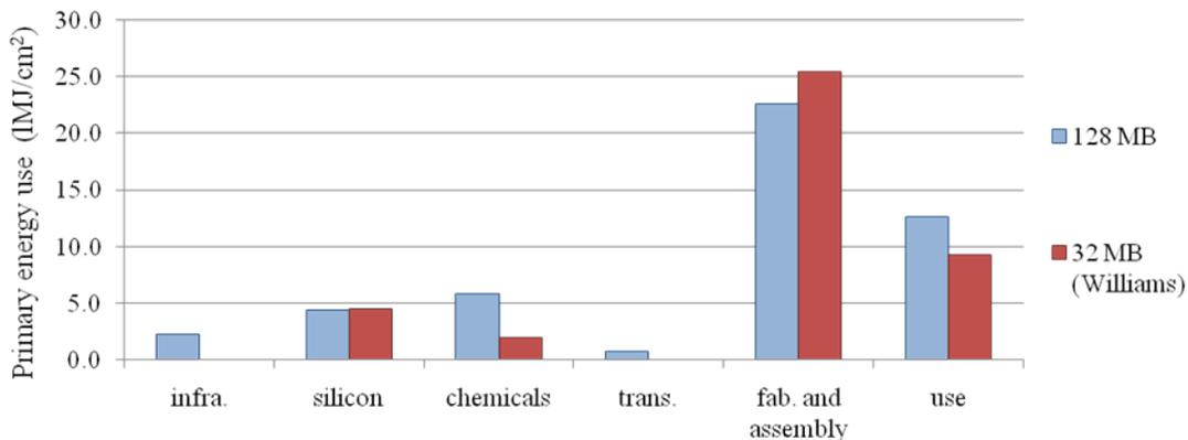
Figure 6.11. Comparison with Williams: Energy use at each life-cycle stage
