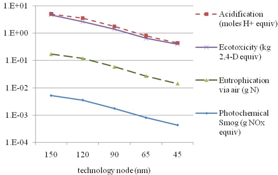
Figure 5.2. Environmental impacts due to air emissions per GB, over five technology nodes
