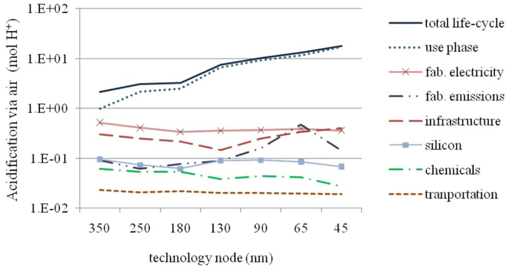
Figure 4.5. Acidification per die by technology node
