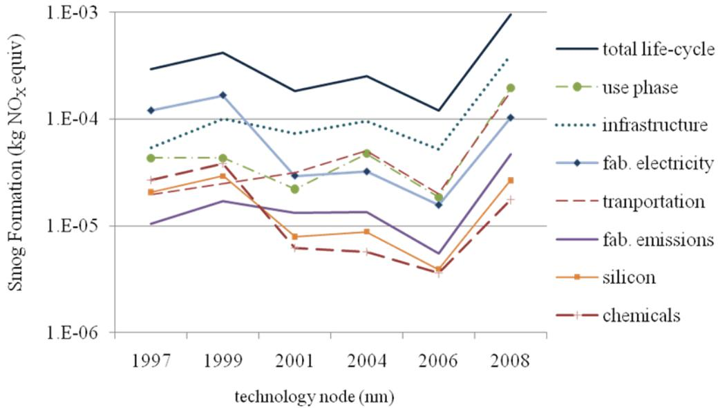
Figure 6.4. Smog formation per OS by technology node
