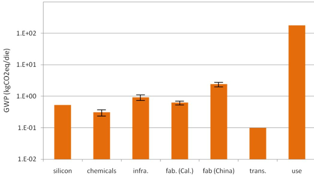
Figure 3.14. GWP of emissions per die by life-cycle phase, 45 nm node
