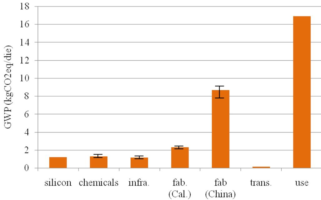
Figure 3.12. GWP of emissions per die by life-cycle phase, 350 nm node
