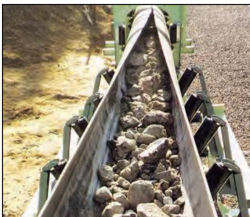
Figures 5.4.3.9.4-2 Typical pipe conveyor. [SRK]
