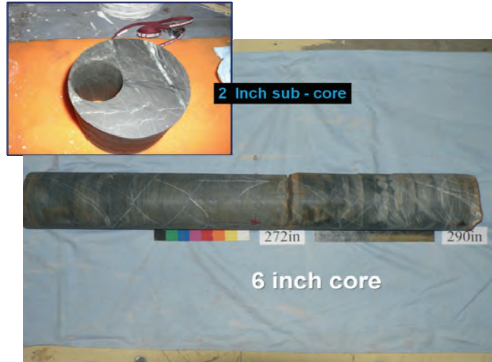
Figure 5.3.2.5-1 Six-inch core preparation for testing. [Golder Associates]
