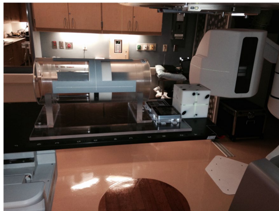
FIG. 4. In-house mount that allows the localization of all phantoms used in the monthly QA in the couch at the same time. In the figure, from left to right we find the Emma, QckV-1, QC-3, and MIMI phantoms.
