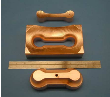
Figure 9. Plunge EDM sample with tellurium copper electrode (bottom) and wire burnout (top).
