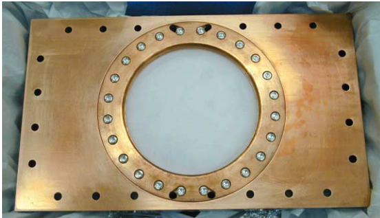
Figure 10. Finished window in waveguide flange.
