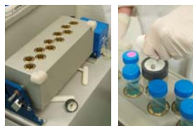
The 'Lock Down' and 'Decapper' tools for removing caps of 50mL conical tubes.
