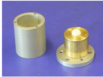
(a) Mechanical Drawing of AR-coating press (b) Photograph of Press with lens
