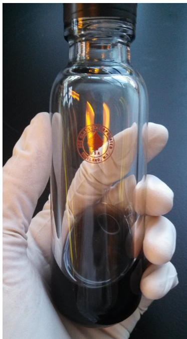
Figure 3.1: Photograph of a vial of organic SWNT ink, containing well-dispersed SWNTs in DMSO without sonication or surfactant.
