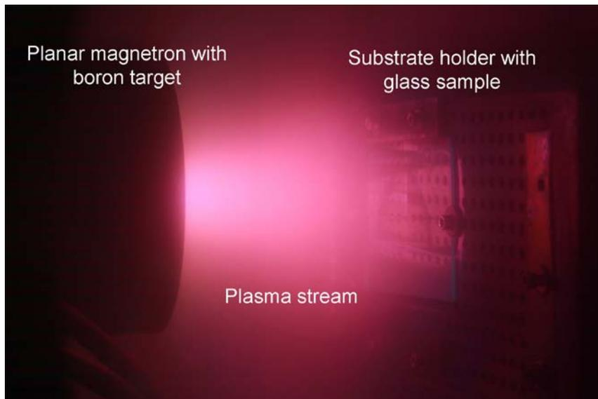
Fig. 2. Photo of the discharge system operating with a pure boron target shown the characteristic red color of the boron-containing plasma. The planar magnetron is to the left and substrate holder to the right, as indicated. Experimental conditions are: nitrogen pressure 1 Pa, frequency 350 kHz, discharge voltage 470 V, average discharge current 0.53 A, average discharge power (power-stabilized mode) 250 W.
