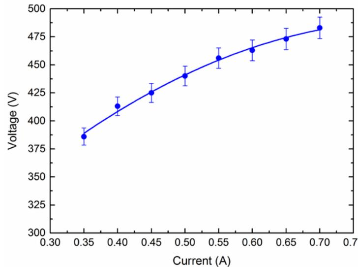
Fig.4. Current-voltage characteristic of a planar magnetron with a boron target; pressure 0.9 Pa (nitrogen), pulse frequency 350 kHz.
