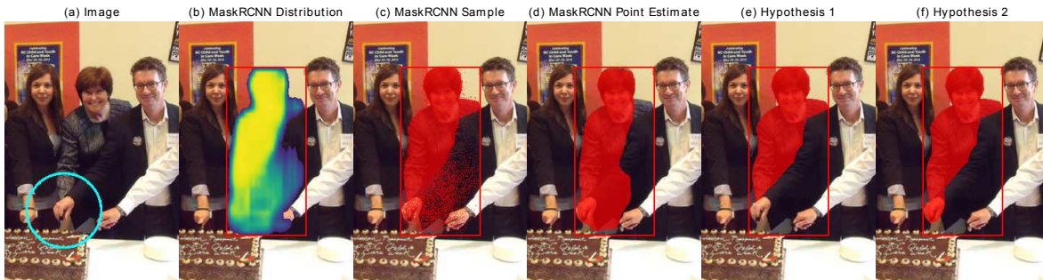
Figure 2.3: In the image shown in (a), who does the hand circled in blue belong to? (b) The pixelwise distribution predicted by MaskRCNN’s mask head, which does not model the dependence between pixels. (c) A sample from this distribution, which independently samples the uncertain pixels in the hand, is not a plausible instance mask. (d) The (incorrect) point estimate that MaskRCNN would return. (e), (f) A more distributionally expressive model might allow us to sample plausible hypotheses like these two. In this case, (e) is actually the correct segmentation.
