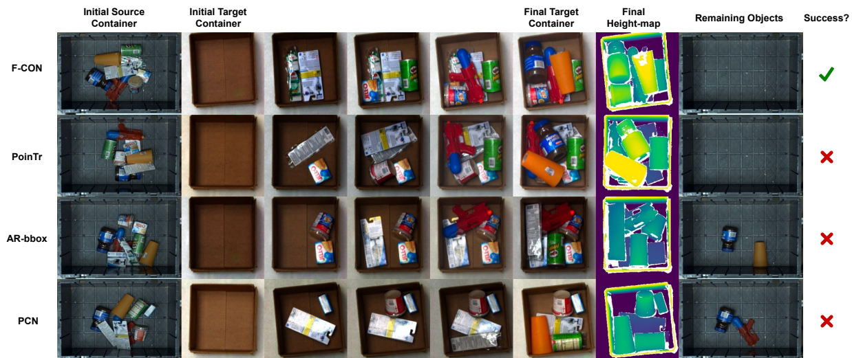
Figure 4.7: Representative episodes from our real-world packing experiments. In each row, we conduct one episode using the listed shape completion model and HM as the planning method. All rows use the same item set. The progress within the episode can be seen from left to right, along with the final height-map. With F-CON (row 1), all of the items can be packed densely. Other methods cause the packing container to overflow (row 2) or they cannot pack all the items (rows 3, 4).
