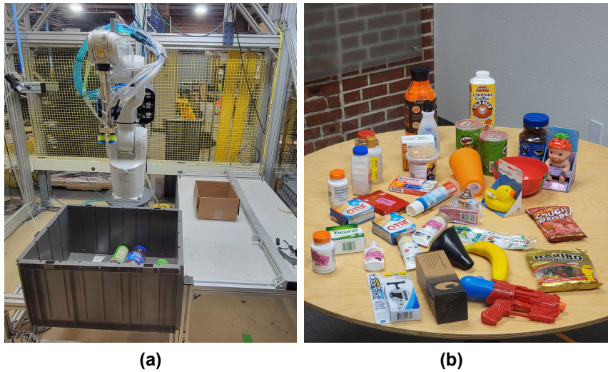
Figure 4.6: (a) Our robot picks items from the cluttered bin in the front, and packs them into the cardboard box on the table. (b) The complete item set used in our experiments.
