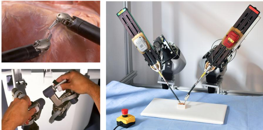
Figure 1.3: Da Vinci Surgical System: (a) Master console along with the visualization system as seen by the surgeon. (Image: Intuitive Surgical) (b) The image depicts the dVRK set-up with two arms at the UC Berkeley Autolab.
