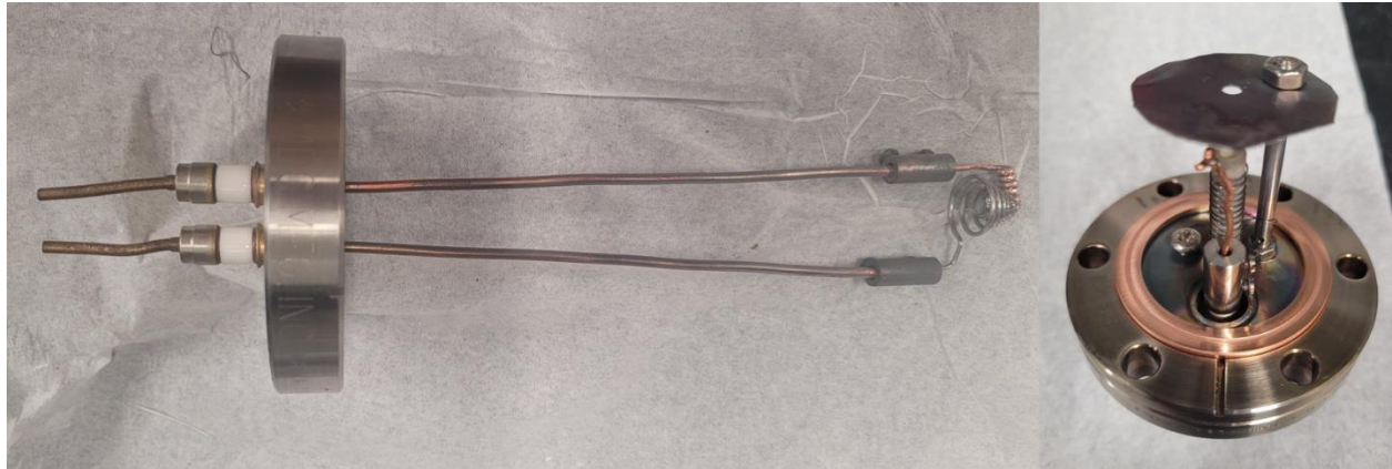
Figure 4.7. Left: Pb evaporator using a tungsten basket design. Right: Pb evaporator using a crucible design.
