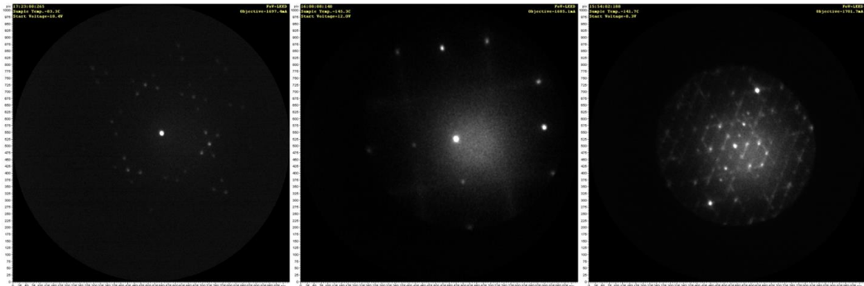
Figure 3.2. LEED Patterns of clean Germanium surfaces, showing Ge(111) c(2x8) at 10.4eV (left); Ge(100) p(2x1) and c(4x2) at 12.0eV (middle); and Ge(110) c(8x10) and (16x2) at 8.3eV (right).
