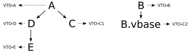
Figure 1.13. The vtable layout inheritance trees of the running example in Figure 1.1
