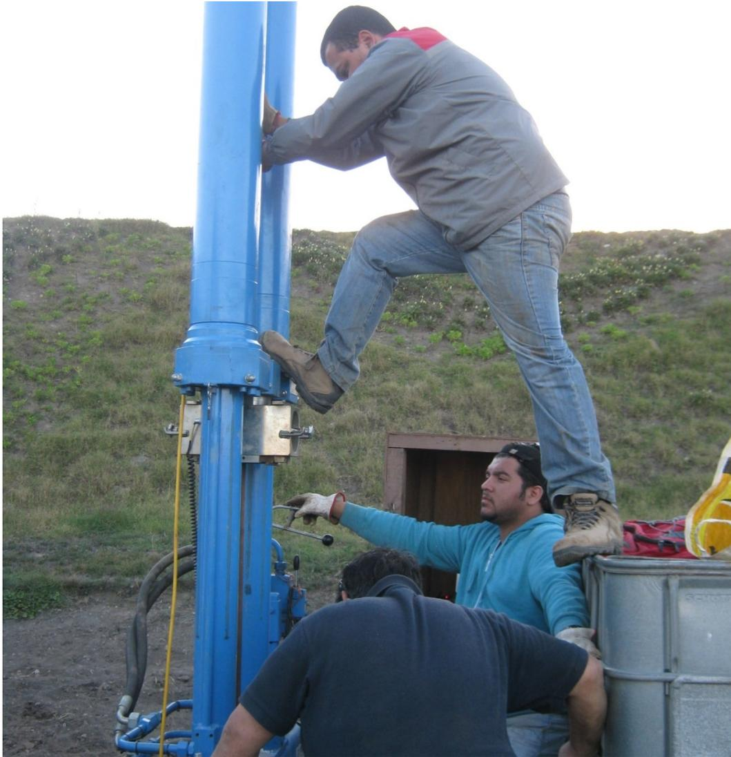
**Fig. 4.5.** IDIEM operators manually shaking the push rods while slowly lowering the hydraulic press to force the clamp grip the push rod
