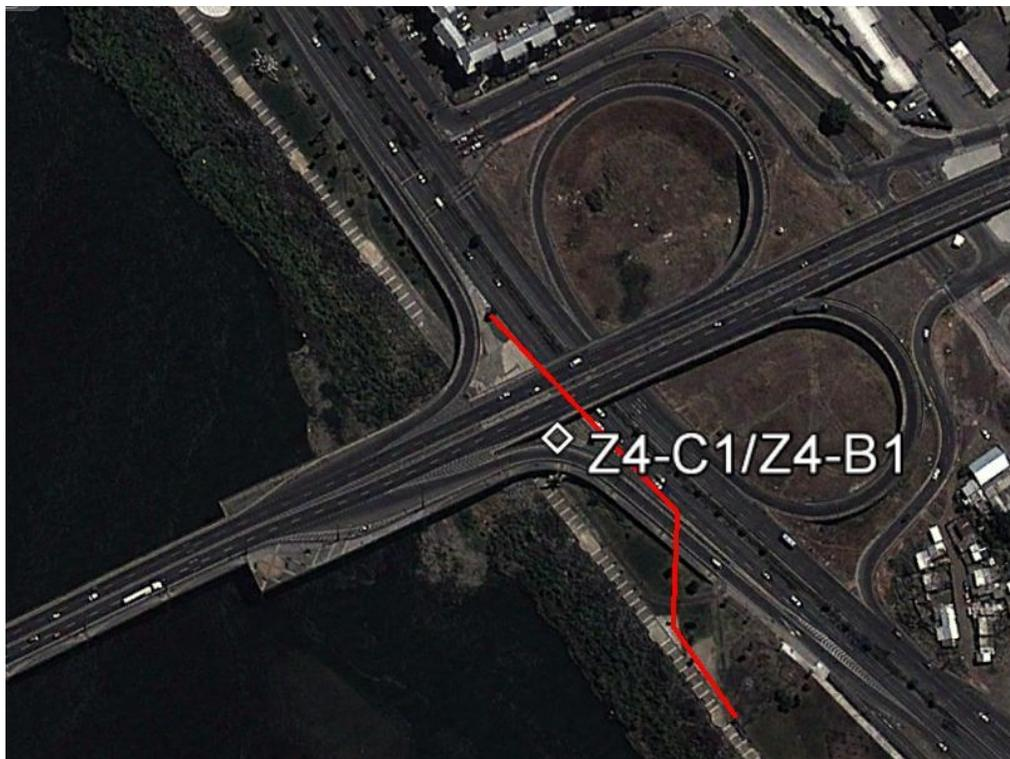
**Fig. 4.28.** Test location with red indicating the extents of lateral spreading observed by GEER
