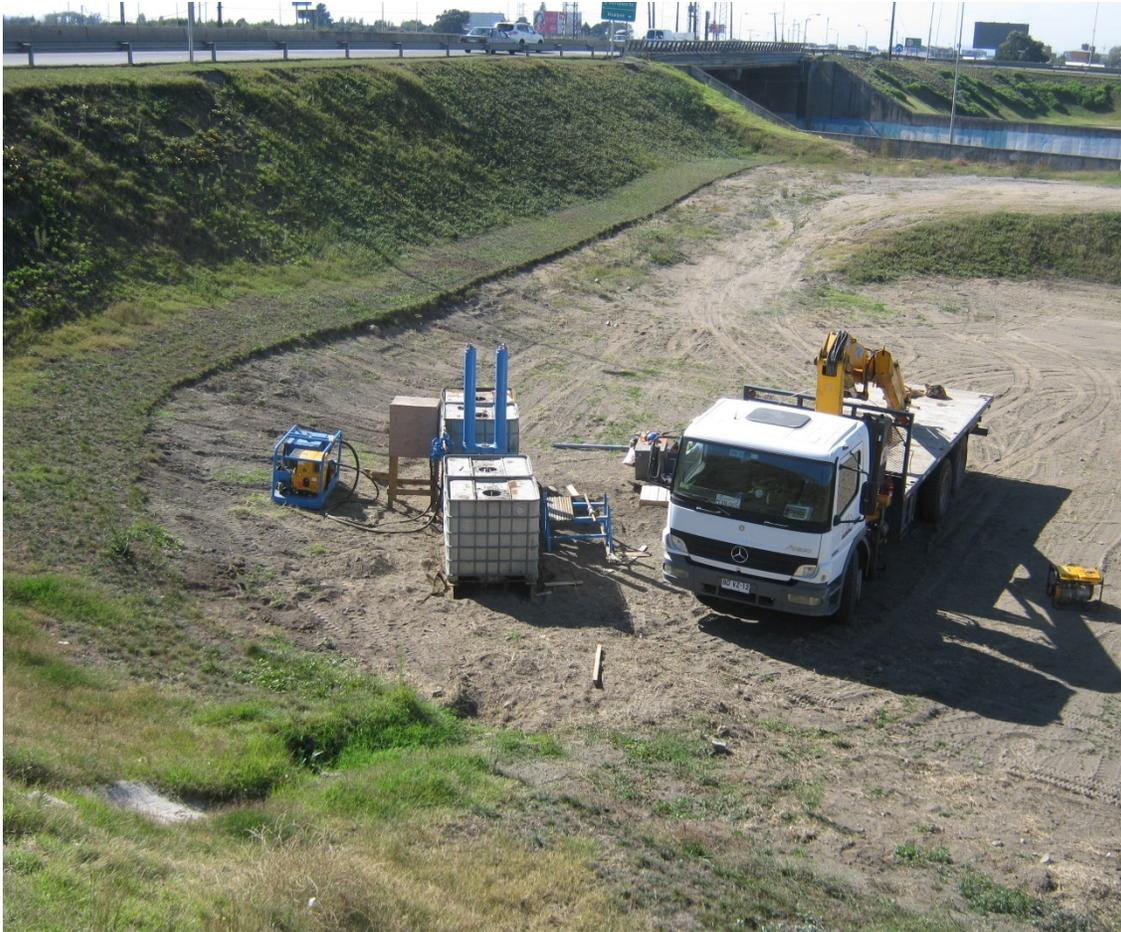
**Fig. 4.25.** CPT Z3-C5 in progress with an area of the highway that suffered liquefaction-induced settlement visible in top left corner
