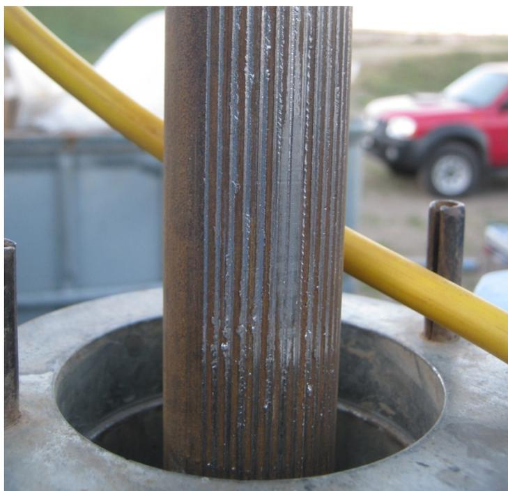
**Fig. 4.4.** Scraped CPT push rod due to insufficient clamp grip
