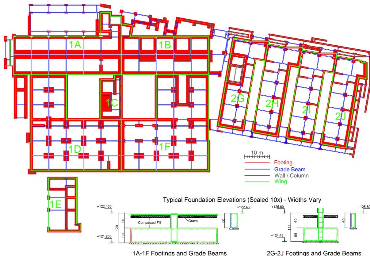
**Fig. 4.9.** Plan view of hospital foundations (foundation measurements in cm)
