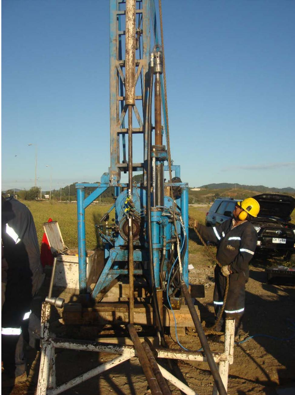
**Fig. 4.7.** SPT performed with energy measurements
