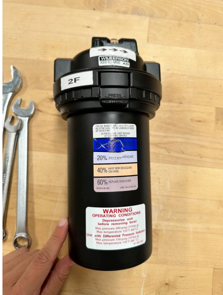
Figure 1: Image of the desiccant bed, from the front, disconnected from system.
