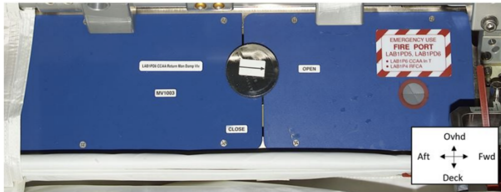
Figure 3. CCAA Return Manual Damper Valve Control Knob, One Each Standoff (LAB1PD6 Shown).
