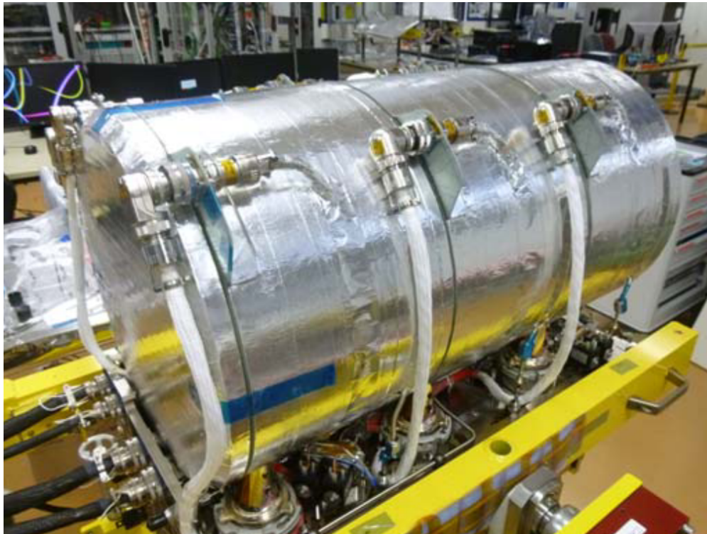
Figure 1.6: Carbon Capture Assembly (CCA) adsorber bed, as shown in literature [7]
