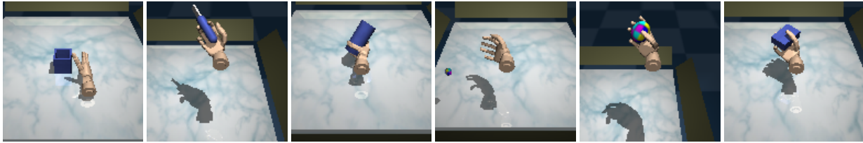
Figure 5.3: Figure showing some of the objects and their grasps by the model (snapshot at different time intervals). Left to right, a can, screw driver, cylinder, coin, ellipsoid and cuboid are shown. The table is bounded by four walls (green in color) that can be seen
