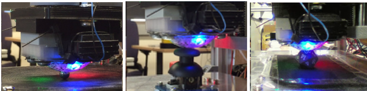
Figure 7.2: We evaluate deep tactile MPC on 3 different fine-grained manipulation tasks: (left to right) ball repositioning, joystick deflection, and die rolling to reach a specified face.
