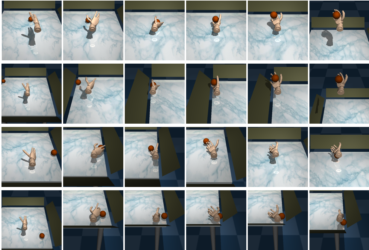
Figure 5.2: Grasp trajectory of a policy learnt to grasp spheres in various initial positions with respect to the hand. The first two rows show cases where the policy succeeds. Left to right, we see the trajectory unroll in six sub images. The general learnt policy is to go under the object and scoop the sphere into the palm. In some cases, it just balances the object in other cases it wedges the object between fingers and sometimes the thumb. The last two rows show cases where the policy fails.
