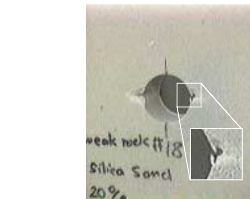
Figure 15. Borehole failure in cemented silica sand bricks
