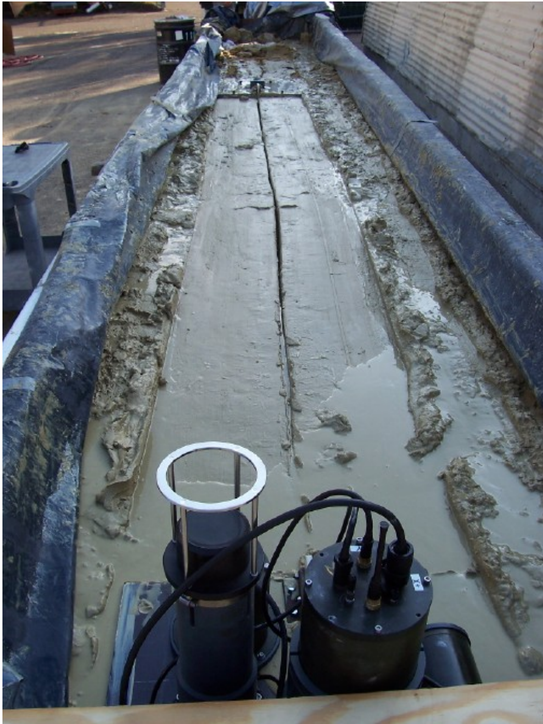
Figure 3.17: Mudpit where we tested the sled. Shown is the rear anchor (foreground), the front anchor (background), and the path of the sled including the trenched fiber.
