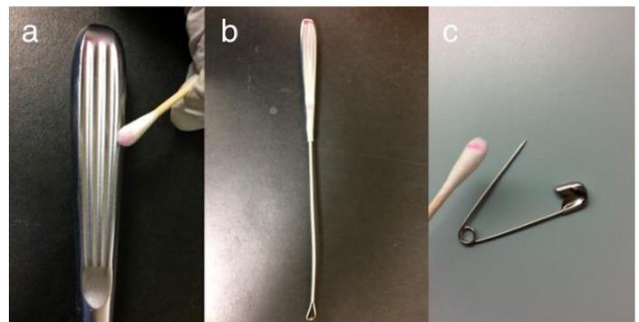
**Figure 4.** Photos **a)** and **b)** of a blunt curette and **c)** of a safety pin, each of which tested positive for nickel release.
