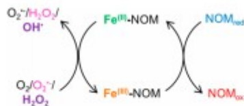
Figure 5. Simplified proposed reaction scheme showing Fe redox cycling in the presence of reduced organic matter and oxygen.
