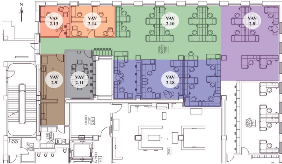
Figure 1.1-5: Temperature control zone plan in Doe Annex
