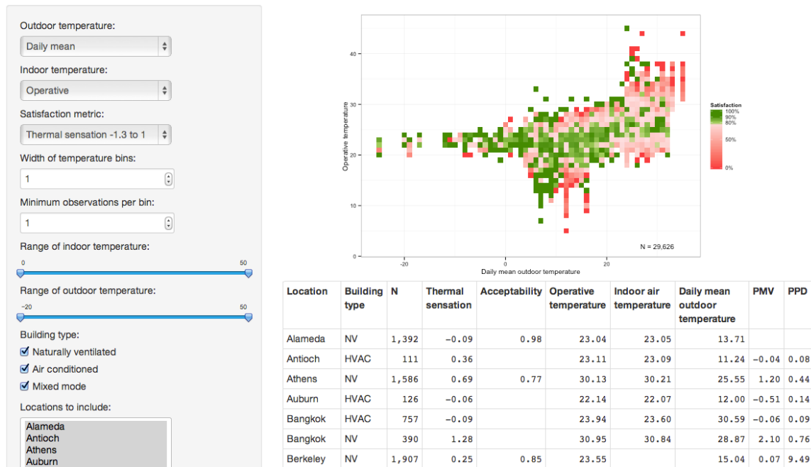
Figure 3.1-2: Mapping tool shows the satisfaction rates on the outdoor vs indoor air temperature map
