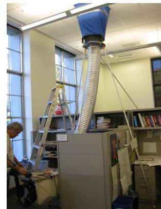
Figure 1.1-6: Airflow calibration process and measured airflow values
