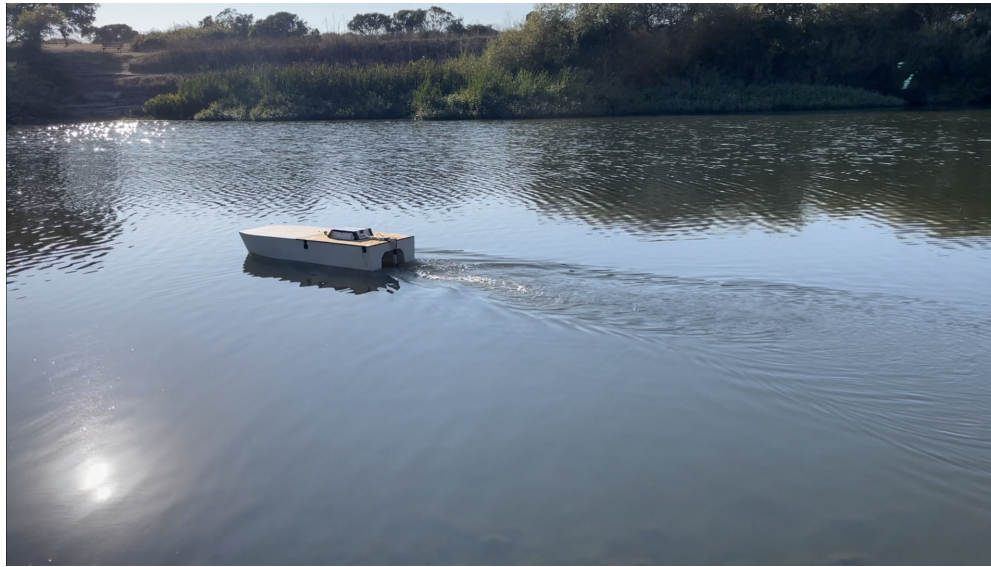
Figure 8.1: The ASV mapping the depth of a freshwater pond in Santa Cruz, California.
