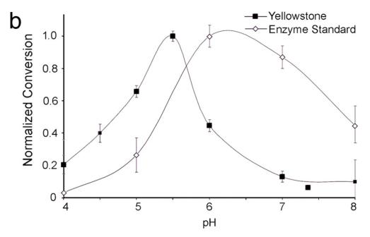
Fig. 6. Direct characterization of the Yellowstone microbial community by using the Nimzyme assay. (a) Screening of the  $\beta$ -galactosidase inhibitors phenylethyl  $\beta$ -d-thiogalactopyranoside and deoxygalactonojirimycin. (b) Determination of optimal pH in the Yellowstone community extracts compared with the  $\beta$ -galactosidase standard. All reactions performed for 15 min in pH 6 ammonium phosphate buffer at 65°C.
