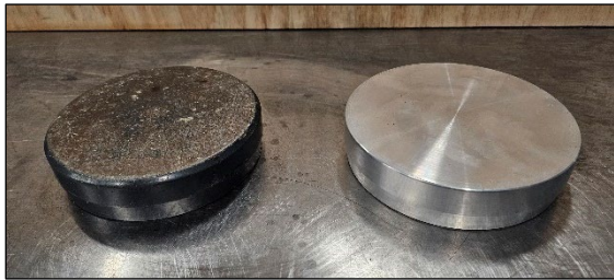
Figure 4.4: Original and new loading platen for Wirtgen cell (new platen on left).
