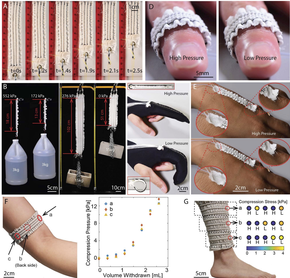
Figure 3.10: Demonstrations. (A,D,E) Miniature soft actuators for linear motion control or compression, capable of (A) lifting a small mass, (D) compressing small tissue areas, or (E) providing tactile feedback via skin stretch. Inset: Skin stretch was easily perceived. (B) FFMS actuators can perform large mechanical work. A 10-channel device lifts a 3 kg mass. A 3-channel structure (inner tube radius 2 cm) lifts a 15 kg cinder block and chain at pressures less than 276 kPa. (F,G) FFMS can be used for compression garments for healthcare, training, and haptics. (F) A compression band yields uniform pressure on the upper limb, easily matching pressures provided by blood pressure cuffs. (G) A compression garment for the lower limb comprises three independently addressable sections (dashed boxes). Pressure variations can yield peristaltic motions suitable for undulatory massage in therapies for lymphatic and blood circulation [69], such as lymphedema [70] or venous closure [71].
