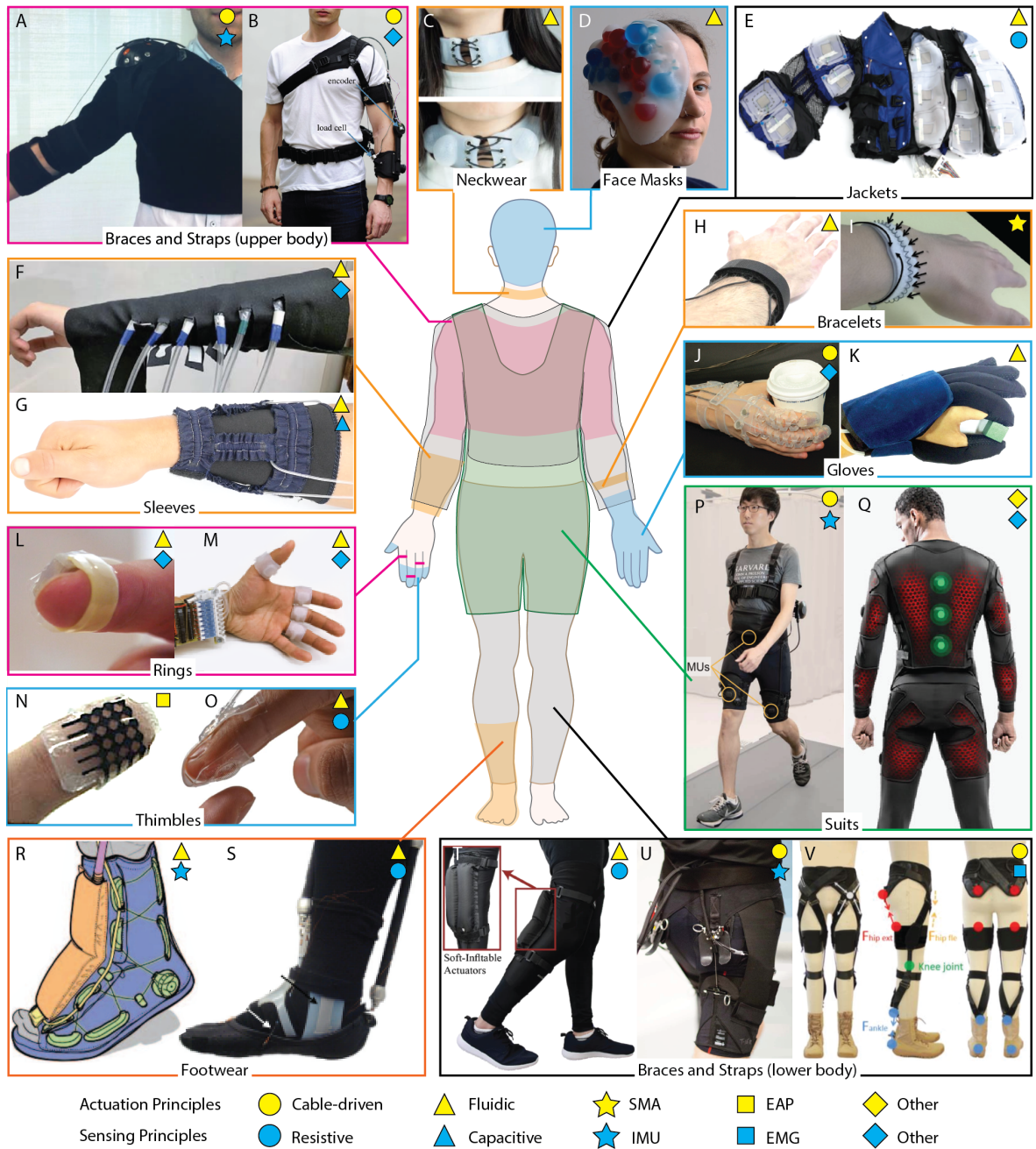
Figure 2.2: Examples of soft wearable robotics and haptic devices in various wearable form factors. Yellow and blue symbols represent different actuation and sensing principles respectively. A-B. Devices consist of braces and straps on the upper body [13, 14]. C. Biometric neckwear [15]. D. Responsive face prosthesis [16]. E. Haptic jackets [17]. F-G. Sleeves [18, 3]. H-I. Bracelets [19, 20]. J-K. Gloves [21, 22]. L-M. Rings on different segments of fingers [23, 24]. N-O. Thimbles [25, 26]. P-Q. Suits [27, 28]. R-S. Footwear [29, 30]. T-V. Braces and straps for lower body [31, 32, 33]. Images reproduced with permission. Images B, C, K are licensed under Creative Commons 4.0.
