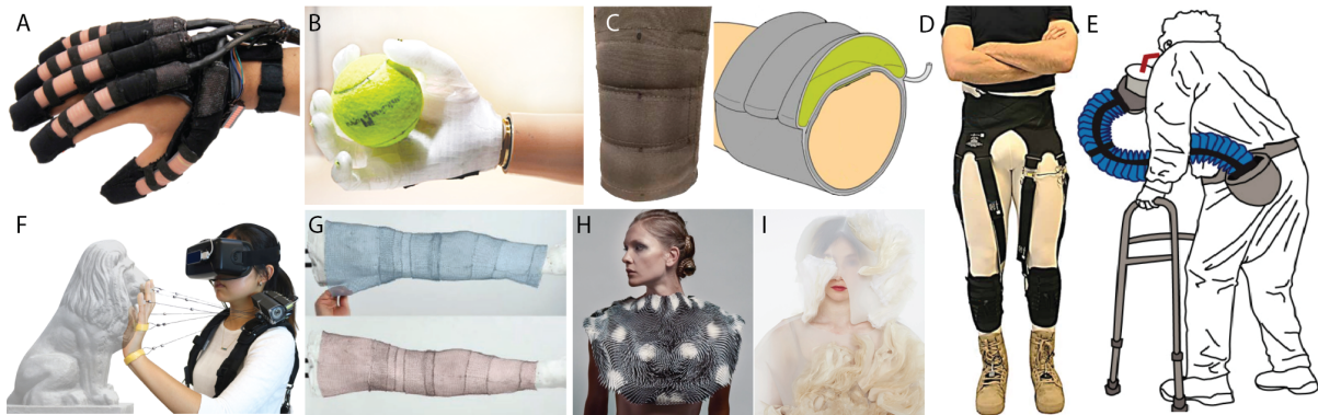
Figure 2.1: Examples of soft wearable devices in diverse application areas. A. Pneumatic glove for hand rehabilitation [4]. B. Cable-driven soft prosthetic hand [5]. C. Segmented pneumatic actuation for compression therapies [6]. D. Cable-driven suit for reducing metabolic costs of walking [7]. E. Supernumerary pneumatic arm for aiding activities of daily living [8]. F. String-based wearable haptic interface for virtual reality [9]. G. Leggings knit from SMA that can contract to match the limb shape [10]. H. Expressive soft robotic garment actuated by SMAs responds to the gaze of others [11]. I. Piezoelectric garment reacts to facial expressions [12]. Images reproduced with permission. Image B is licensed under Creative Commons 4.0.
