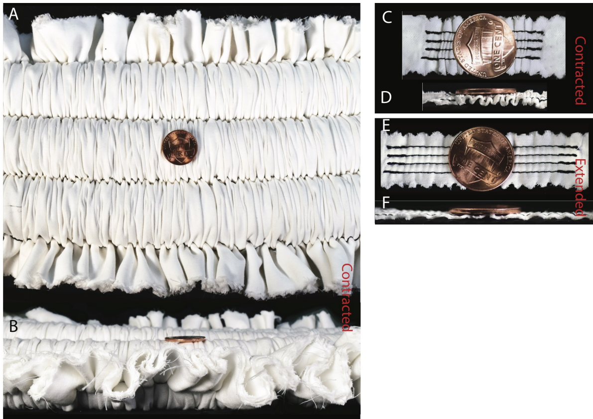
Figure 3.8: FFMS actuators are readily scaled to small and large sizes. (A,B) A large example, consisting of a 34.0 mm thickness FFMS (A: Top view, B: Side view), shown in contracted state, was sufficient to lift 15 kg (Fig. 3.10). (C-F) A small example, in contracted (C,D) and extended (E,F) states; the thickness when extended is 1.0 mm. The large and small actuators were fabricated using the same general process. A penny is used to illustrate the relative scale.
