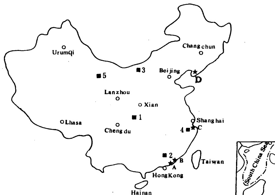
Figure 6.1. Map showing distribution of nuclear power plants (NPPs) on Chinese mainland. Legend: A - Daya Bay NPP; B - Lin'ao NPP; C - Qinshan NPPs (Phases 1, 2, and 3); and D - Liaoning NPP. Preselected regions for development of HLW repository: 1 - southwest China (granite, shale); 2 - Guandong area (granite); 3 - Inner Mongolia (granite); 4 - east China (granite, tuff); and 5 - northwest China (mudstone, shale, granite).
