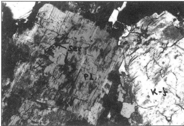
Figure 13.2. Plagioclase feldspar (P1) and K-feldspar (k-f), filled with sericite in a thin section of granite. Network of microcracks are also observed. Under crossed polars (x16).
