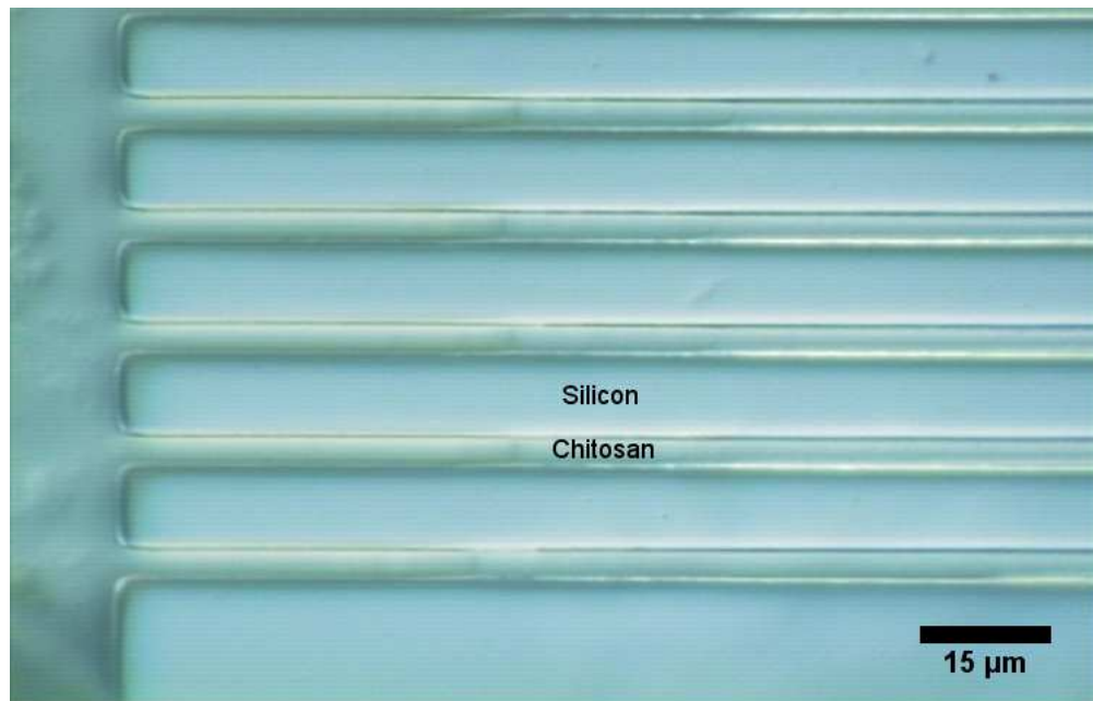
Figure 2.16: Chitosan following lift-off of patterned photoresist using PRS-3000
