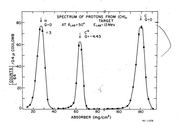
Fig. 5. Differential range spectrum of protons from CH target at  $\theta_L$  = 50°.
