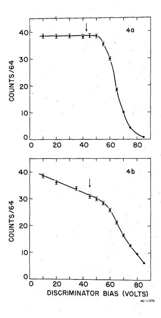
Fig. 4. Typical discriminator curves. A is for counter No. 1 with biases on counters No. 2 and No. 3 fixed. B is for counter No. 2 with biases on counters No. 1 and No. 3 fixed. Arrows indicate bias levels chosen for operation.
