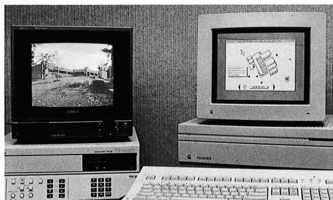
A prototype workstation for advanced computer-based building design. A simulated video building tour can be conducted through a moving icon on plan drawings.
