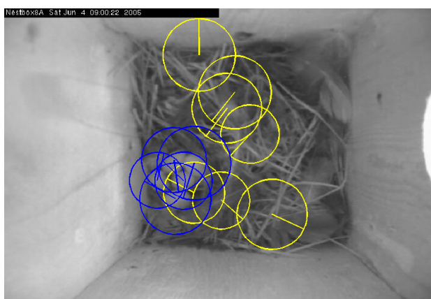
Figure 11. The SIFT features found for an example image of 5 eggs. Blue marks indicate SIFT features corresponding to eggs.
