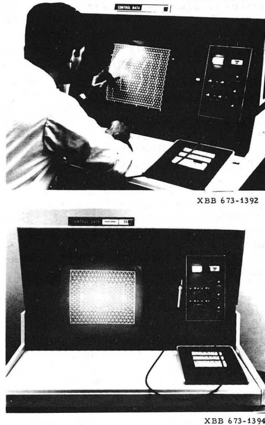
Fig. 4. (a) Preparation of mesh on the console. (b) Final generated mesh.
