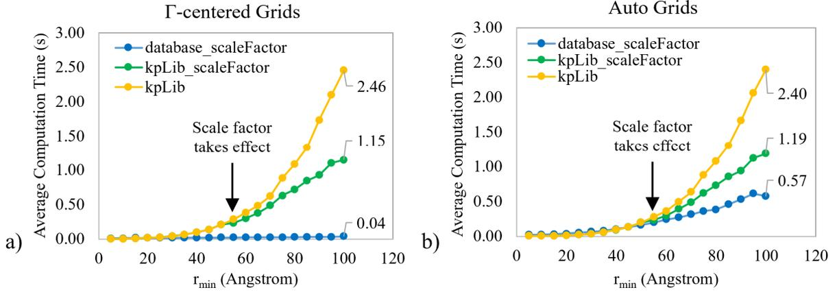
Figure 7. Comparison of computation time between database lookup method used by the  $K$ -Point Grid Generator and the dynamic generation approach used by kpLib. This benchmark did not include monoclinic and triclinic structures, as both the  $K$ -Point Grid Generator and kpLib use dynamic grid generation for these.
