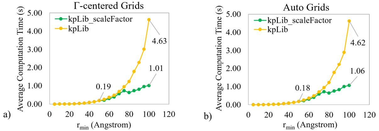
Figure 6. Average computation time of dynamic generation using kpLib with and without scale factors at various values of  $r_{min}$  for a)  $\Gamma$ -centered grids and b) auto grids. The computation times at  $r_{min} = 100$  angstroms are labeled on the graphs.
