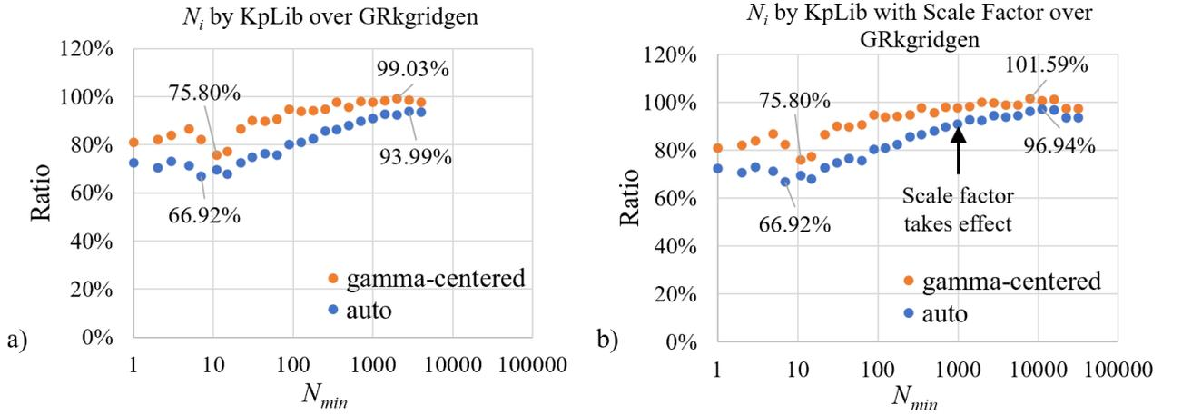
Figure 8. Ratios of average number of symmetrically irreducible  $k$ -points from the dynamic search by a) kpLib, b) kpLib with the scale factor, to grids generated using GRkgridgen, for both  $\Gamma$ -centered grids and auto grids. Both the maximal and minimal ratios are labeled for both types of grids. Part b) has a larger range of  $N_{min}$  (from 1 to 15,848), to better demonstrate the effect of the scale factor on grid quality.
