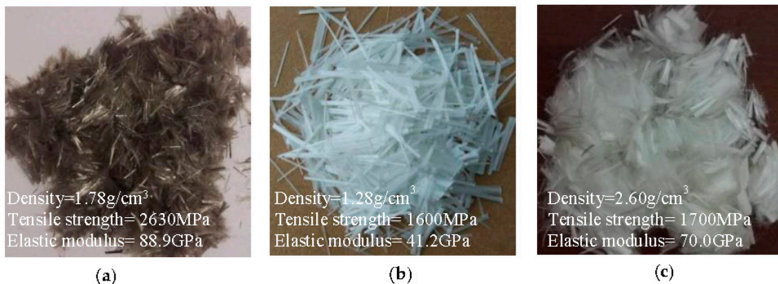
Figure 1. Three types of fiber: (a) basalt fiber, (b) polyvinyl alcohol (PVA) fiber, and (c) glass fiber.
