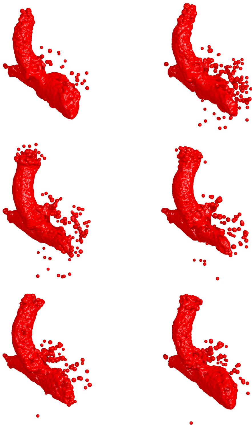
Figure 3.19: Simulation results with mesh interpolation disabled, for comparison purposes. The larger number of leaked particles is noticeable.
