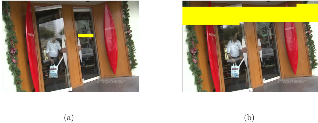
Figure 2.7: Examples of one IP packet loss: (a) one IP packet loss in I frame (b) one IP packet loss in P frame.
