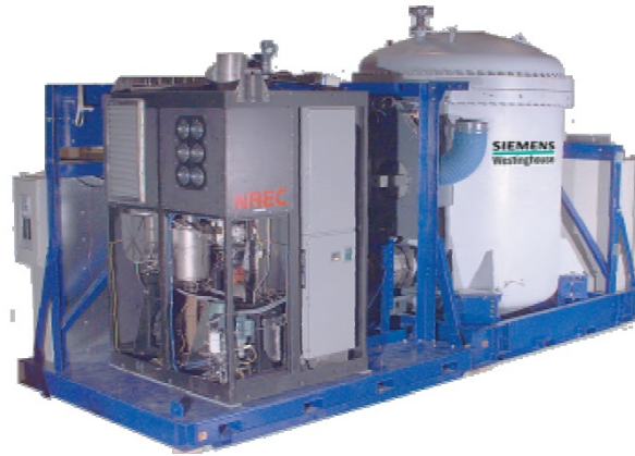
Figure 2.21: Pressurized 220 kW SOFC/Gas Turbine Hybrid [30]
