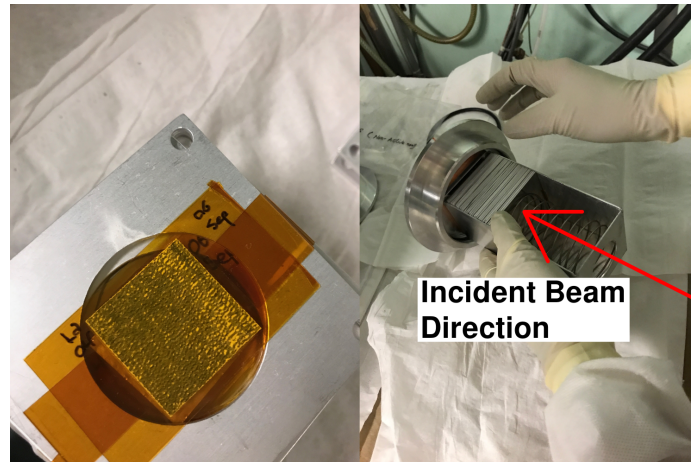
FIG. 1. Photo of an individual foil packet secured to the aluminum sample holder (left) and the entire foil stack (right). The front of the stack (facing the beam) is oriented towards the right in this photo.
