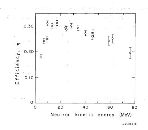
Fig. 9. Total efficiency for detecting neutrons. O Theta zone No. 5.  $\Delta$  Theta zone No. 2.
