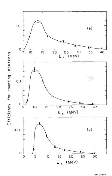
Fig. 8e, f, g. Neutron counting efficiency  $\eta$  as a function of incident neutron kinetic energy  $E_{\bf n}$ , for (e) time bin 5, (f) time bin 6, (g) time bin 7.
