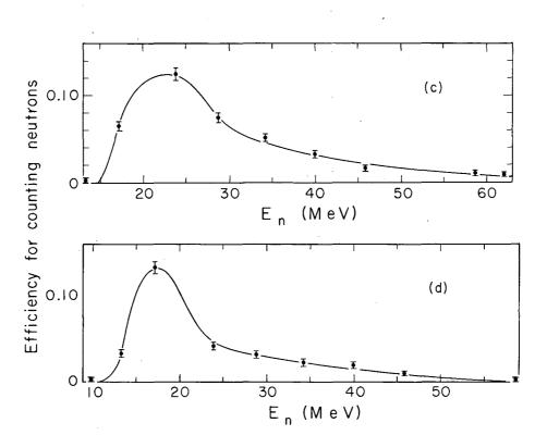
Fig. 8c,d. Neutron counting efficiency  $\eta$  as a function of incident neutron kinetic energy  $\boldsymbol{E}_{n}.$
