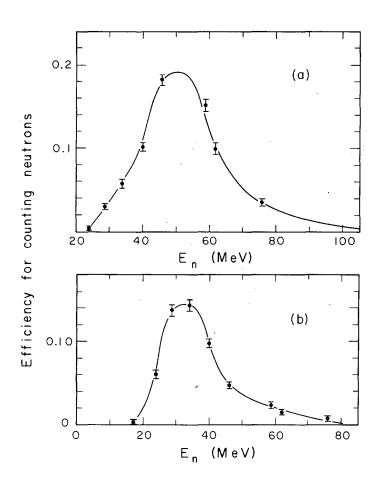
Fig. 8a, b. Neutron counting efficiency  $\eta$  as a function of incident neutron kinetic energy  $\boldsymbol{E}_{\boldsymbol{n}}.$
