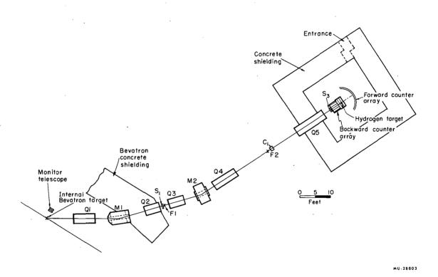
Fig. 2. Diagram of the magnet system and counter placement.
