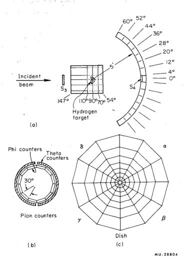
Fig. 3. Geometric arrangement of counters. The side view is shown in (a). Front views of the pion counters and the dish are shown separately in (b) and (c). (View as seen looking along the incident beam).
