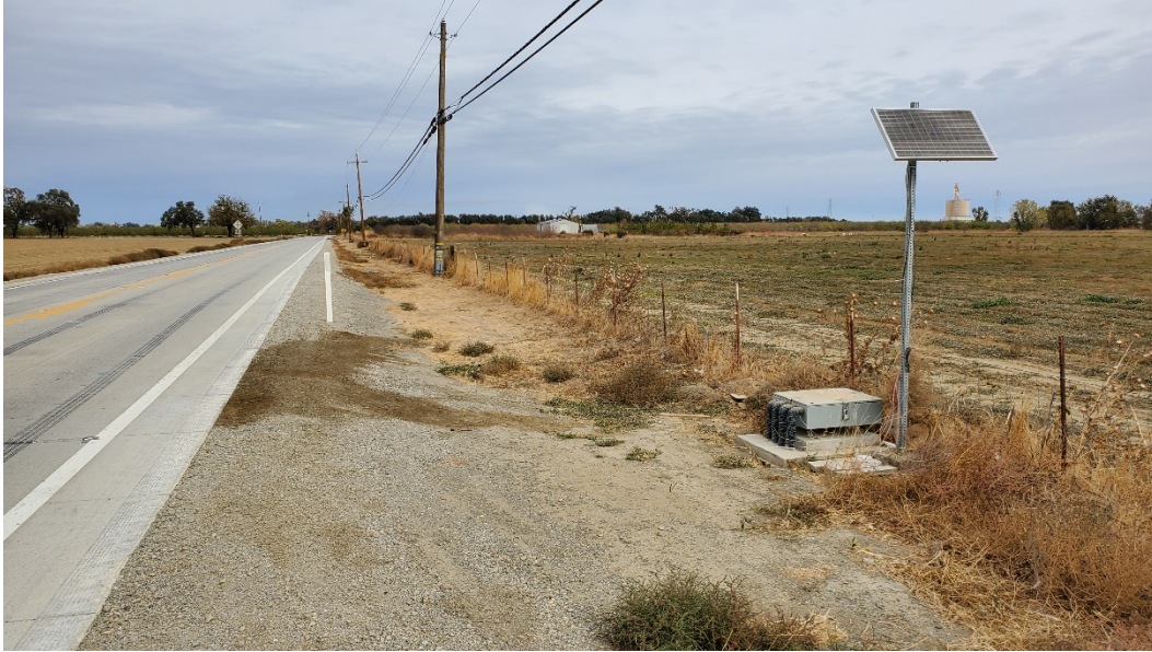
Figure 3.3: Fixed DAS set up to collect hydrothermal data from IPs A21, A22, and A31.
