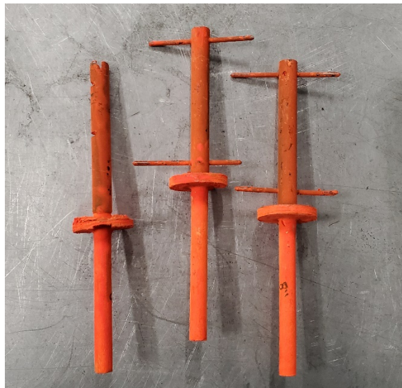
Thermocouple rod (left), strain gauge rods (center and right)
