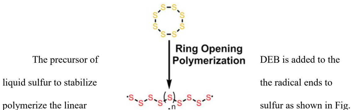
Fig.4. 1 Illustration to ROP of Elemental Sulfur
