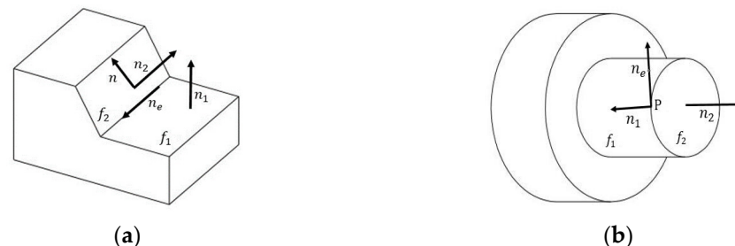
Figure 8. Concavity–convexity judgment of model edge. (a) shows the intersection line of two planar planes; (b) shows the intersection line of planar plane and curved surface.
