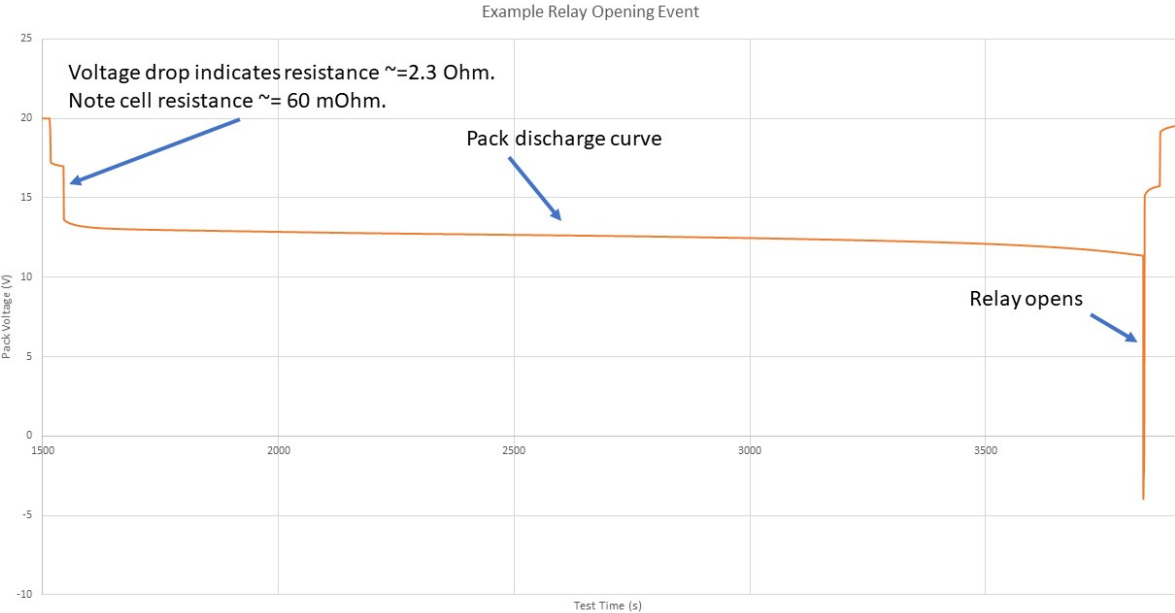
FIGURE 27. Plot of pack voltage over a discharge cycle, showing the relay cutting off the discharge step.
