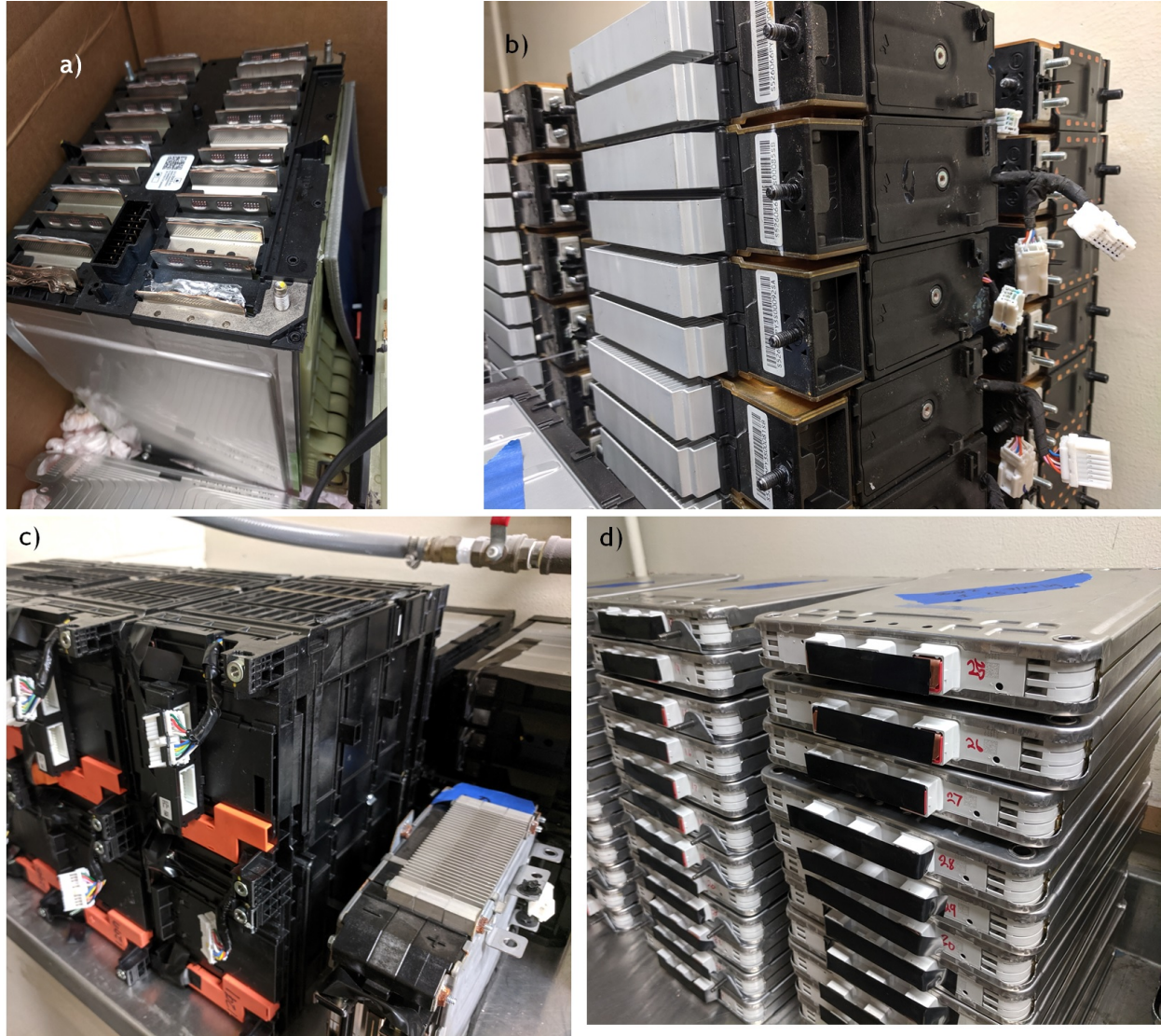
FIGURE 6. Figure showing battery modules from different electric and hybrid electric vehicles. a) Chevy Volt battery module. Note the cooling plate can be seen in the bottom of the image, along with the coolant distribution system at the bottom right. b) Hyundai HEV battery modules. The aluminum heat sink that can be seen of the left side of the modules formed a duct within the pack that was attached to a blower fan. c) A different Hyundai HEV battery module with a smaller heat sink assembly. d) Second gen Nissan Leaf battery modules, which had no integrated thermal management system.
