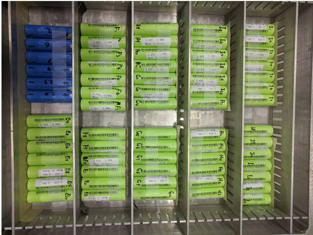
FIGURE 20. Image showing a sample of the cells in an NR imaging tray. For through-axis images, cells were taped to the divider to be held vertically in the tray.
