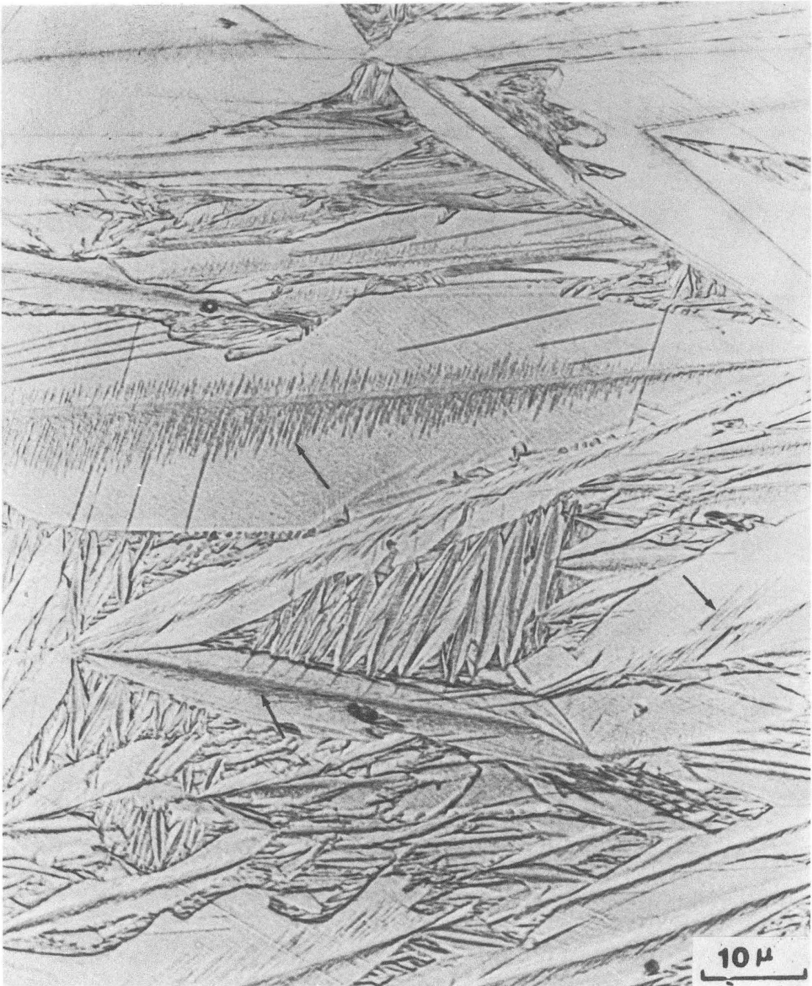
Fig. 8 Magnified image of twinned plates of alloy T showing twin markings (indicated by arrows).
