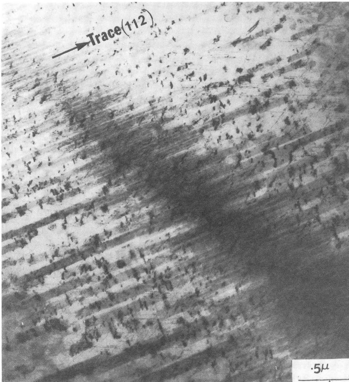
Fig. 17 Steel TC quenched and tempered at 200°C, showing nucleation of carbide (cementite) at the twins. The twin traces are faintly visible and are identified as (112) Traces.
