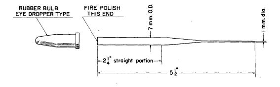
Fig. 2 shows the pipette utilized in the removal and transfer of the lipoprotein-containing top fraction from the preparative tube.
