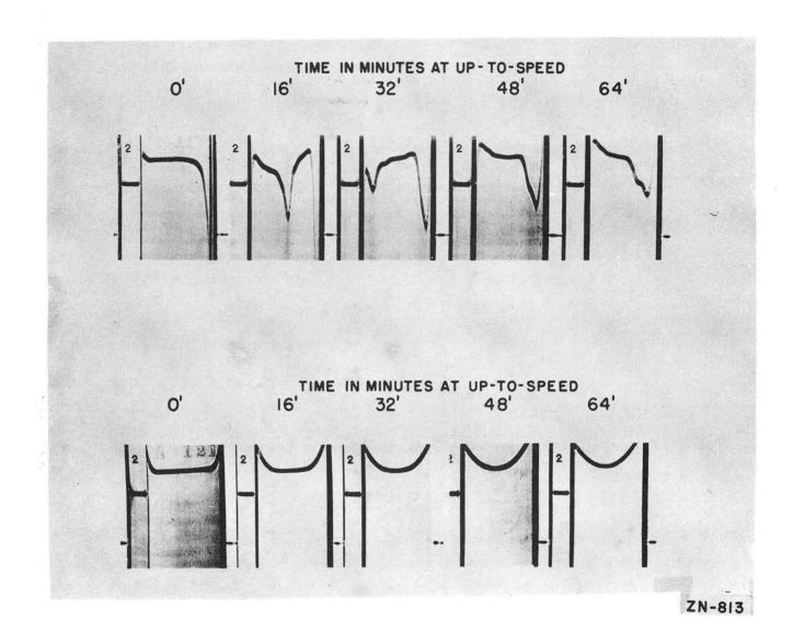
Fig. 12(a) is an analytical ultracentrifugal film record showing the lipoproteins observed in a human specimen at solution density 1.20 gms/ml (Prep Type 3) Rotor speed = 52,640 RPM
