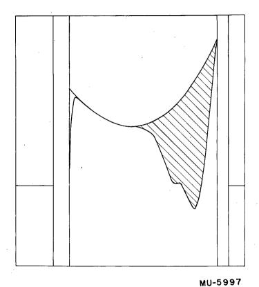
Fig. 13 shows the enlarged tracing used and the area measured in the determination of the sum of the concentration of the lipoprotein of 1.075 gms/ml and 1.145 gms/ml. The tracing represents the 64 minute UTS exposure of Fig. 12 (a) with its superimposed salt reference tracing:
