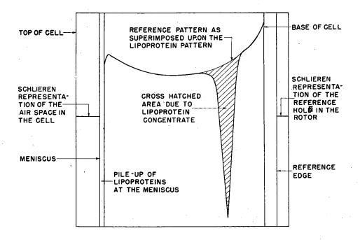
Fig. 5 is a schematic representation of the 30 minute UTS exposure of Fig. 4(a) with the reference baseline of the corresponding exposure of Fig. 4(b) superimposed.
