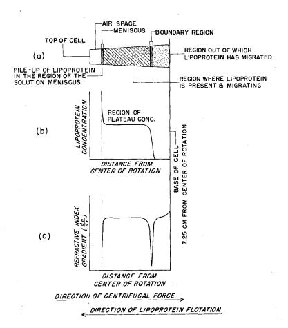
Fig. 3 (a) is a schematic diagram of the analytical ultracentrifuge cell containing a migrating lipoprotein species.
