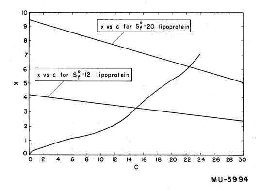
Fig. 8(b) shows the integral curve (representing the cross hatched area of Fig. 8(a) )superimposed on a template inscribed with the s versus o dependence plot for the  $S_f^012$  and  $S_f^020$  lipoproteins. The plotted points of the integral curve represent cumulative sums of the ordinates of Fig. 8(a) at successive equal intervals along the x axis. An ordinate in Fig. 8(a) equals the vertical distance between the lipoprotein pattern tracing and that of the salt reference tracing.
