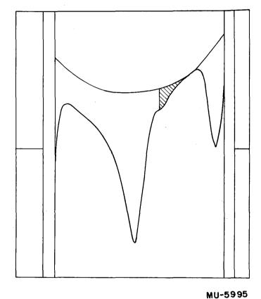
Fig. 10 shows the enlarged tracing used and the area actually measured in determination of the lipoprotein of hydrated density 1.05 gms/ml. The tracing represents the 32 minute UTS exposure of Fig. 9(a) with its superimposed salt reference tracing.
