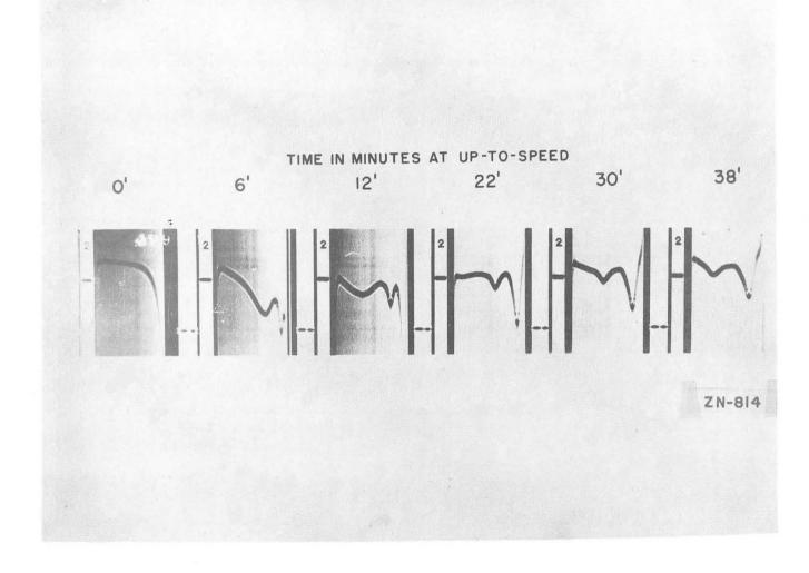
Fig. 6 is an analytical ultracentrifugal film record, demonstrating the various lipoprotein species commonly present in human serum. The lipoprotein concentrate for this run was obtained by preparative procedure Type 1. (Solution density 1.063 gms/ml at 26°C) Rotor speed = 52,640 RPM
