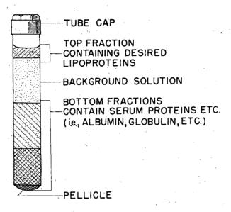
Fig. 1 shows the distribution of serum components in the preparative tube upon completion of the preparative ultracentrifugal run.
