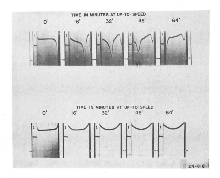
Fig. 9(a) is an analytical ultracentrifugal film record showing the lipoproteins observed in a human serum specimen at solution density 1.125 gms/ml (prep Type 2) Rotor speed is 52,640 RPM.
