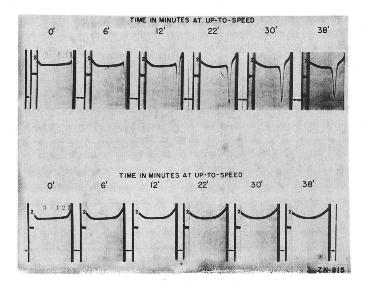
Fig. 4(a) is an actual analytical ultracentrifugal film record demonstrating a single lipoprotein species undergoing flotation in a medium of solution density 1.063 gms/ml at 26° C (Prep Type 1)(52,640 RPM)
