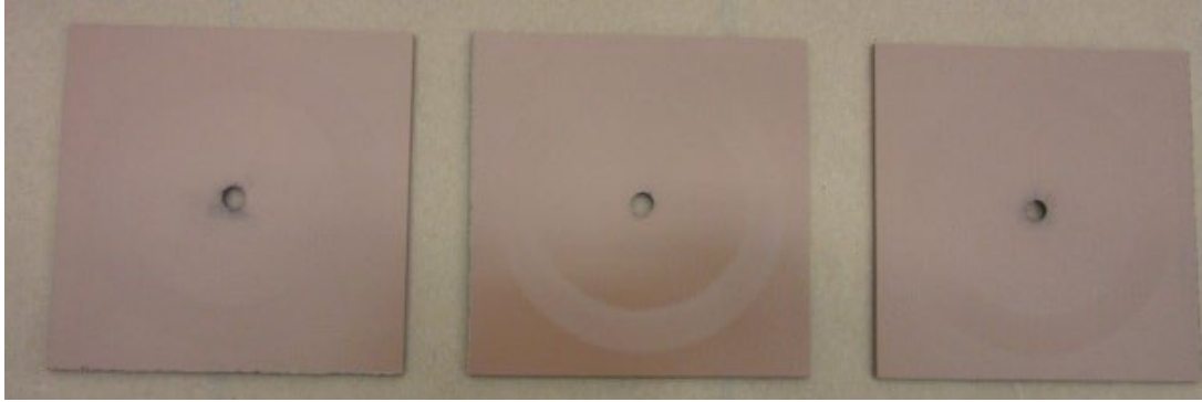
Figure 43: Coated composite panels after abrasion testing
