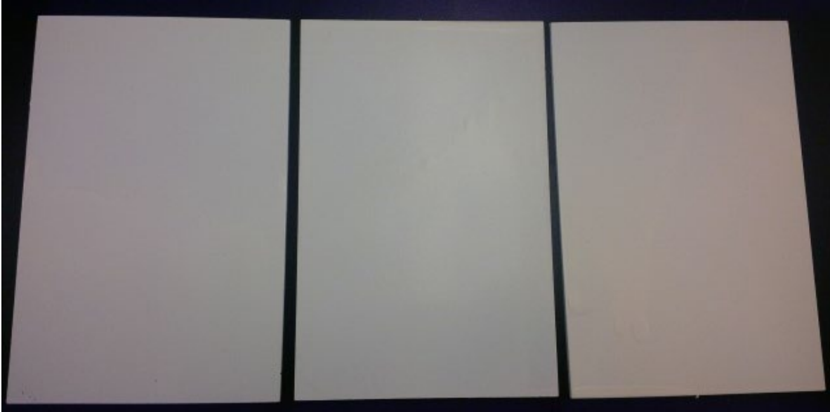
Figure 22: Thermal Cycling Resistance – Coating 3
