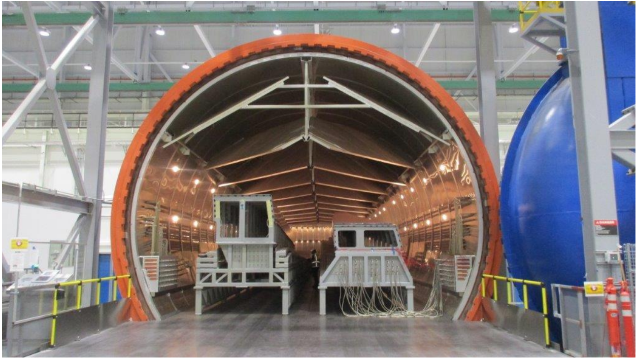
Figure 1: Composite autoclave and lay-up cure tool
