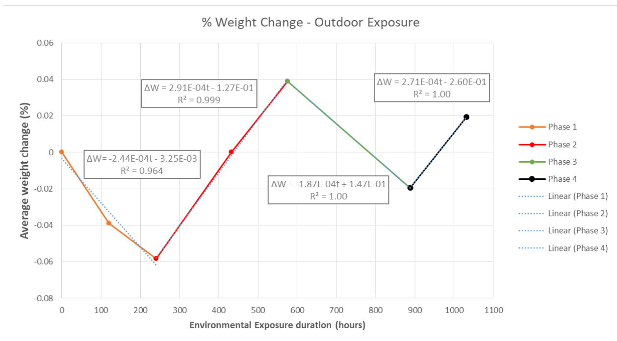
Figure 40: Environmental Exposure duration (hours) vs. Percent Weight Change linearly fit in four phases
