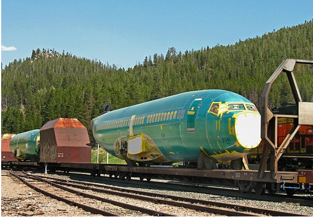
Figure 6: Protective coating utilized to prevent corrosion on metal airplane parts during transport
