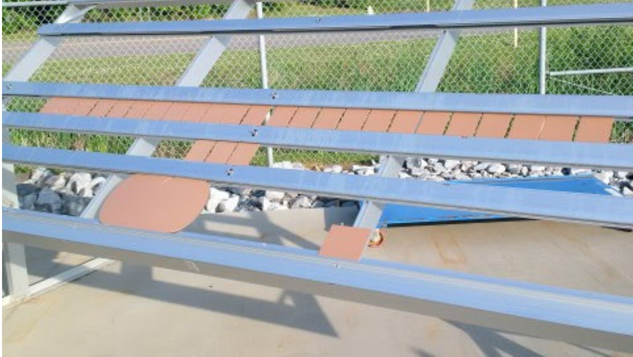
Figure 33: Coated composite panels on Outdoor Exposure rack
