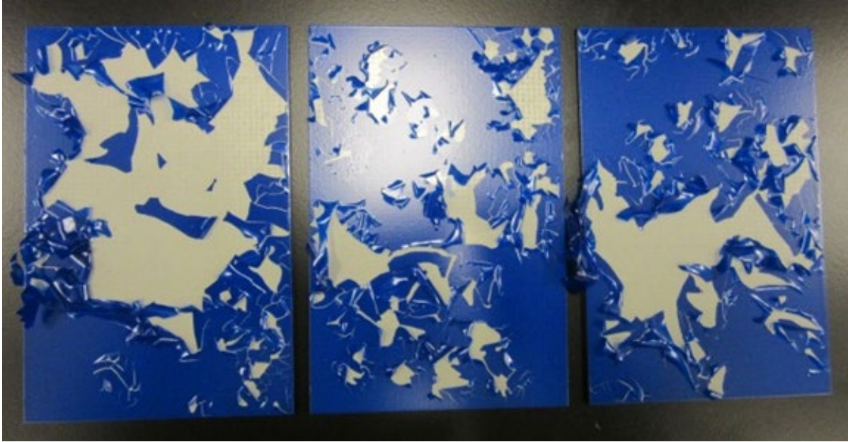
Figure 20: Thermal Cycling Resistance – Coating 1
