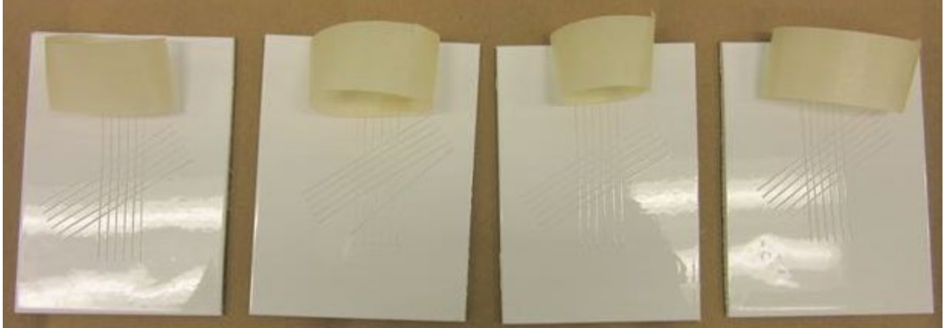
Figure 58: Adhesion testing of composite panels coated with protective coating and an assembly topcoat after UV light and water exposure
