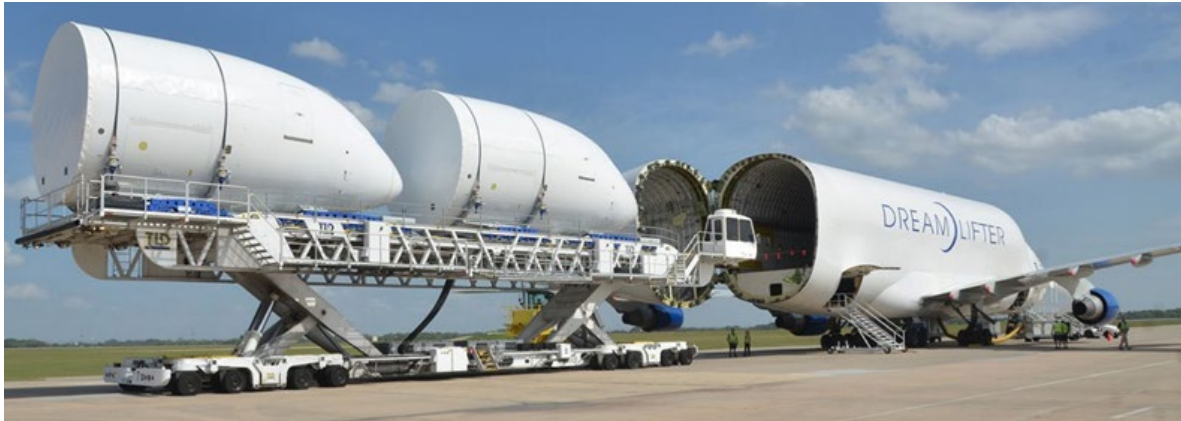
Figure 5: Protective coverings used for composite parts during transport
