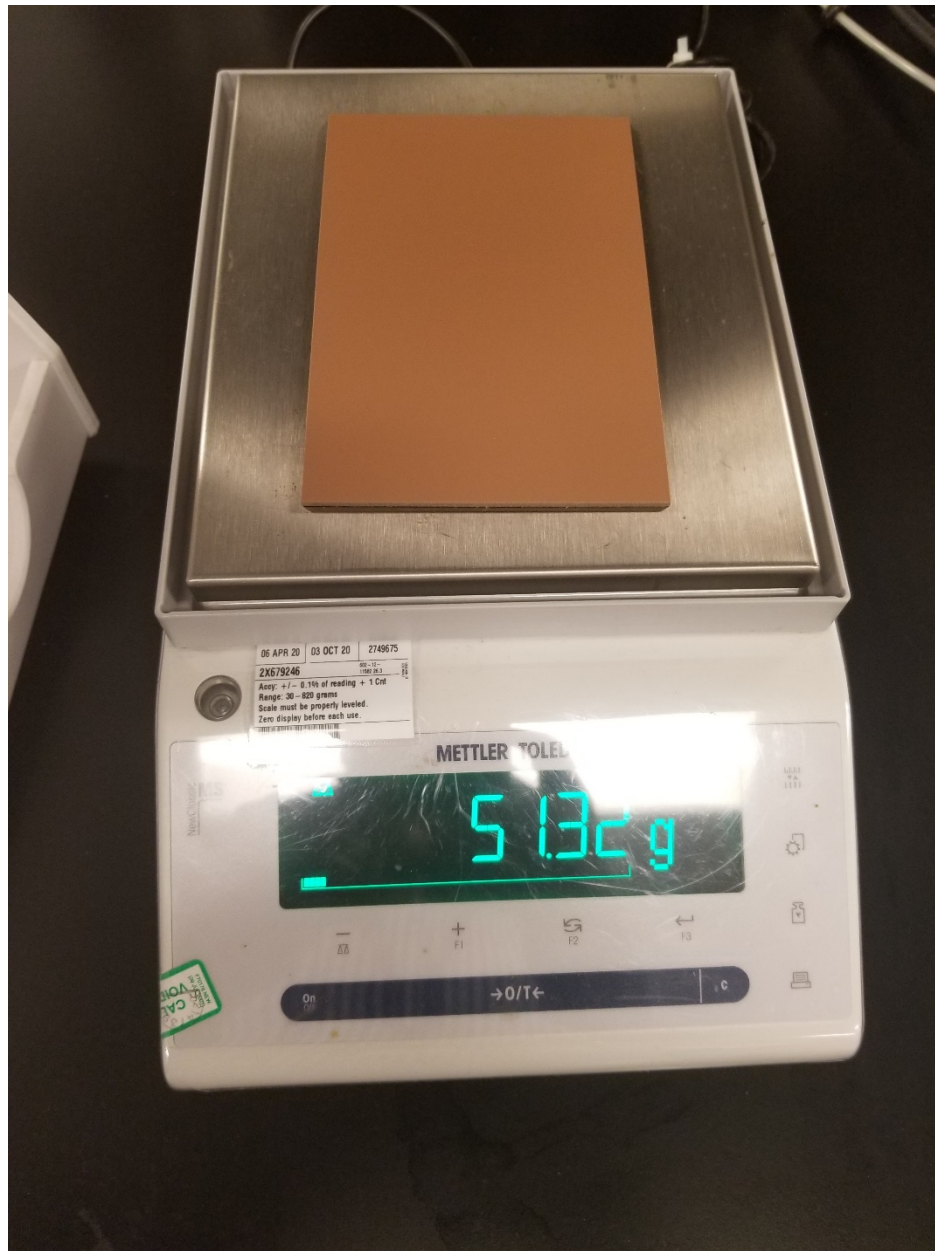
Figure 28: Coated composite test panel being weighted on an analytical balance
