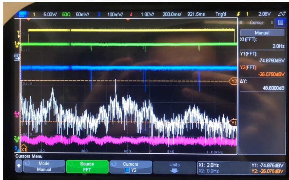
Figure 3.15 Double locking and feedback signal frequency spectrum
