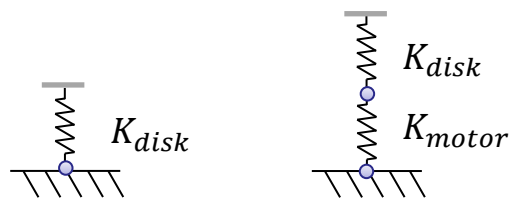
Figure 5.13: Schematic diagram showing the effect of motor flexibility
