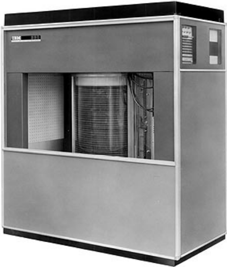
Figure 1.4: The first hard disk drive - IBM 305 RAMAC [IBM]
