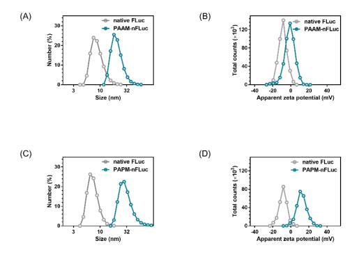
Figure 3-8 The size and zeta potential distribution of PAAM-nFLuc and PAPM-nFLuc. (A)
