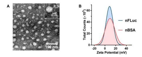
**Figure 2-5 Comparison of nBSA and nFLuc. (A)** TEM images of BSA nanoparticles encapsulated with the same procedures indicating the same morphology with nFLuc(6mV). **(B)** Comparison of zeta potential of nBSA and nFLuc with the same procedures.
