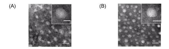
Figure 3-7 TEM images of PAPM-nFLuc (A) and PAAM-nFLuc (B).
