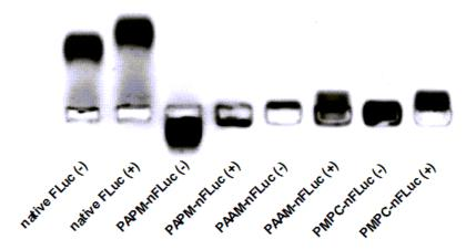
Figure 3-6 Stability of nFLuc nanocapsules against heparin competition for 30 mins via agarose gel electrophoresis.
