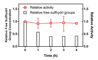
Figure 3-5. Average number of remained thiol groups quantified by Ellman's assay and relative residual activity for 4 hours post reaction.
