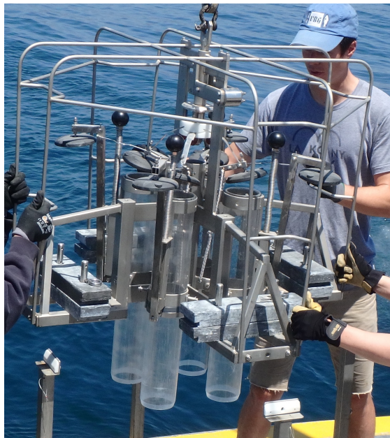
Figure 2-3: Sediment multicorer. The MUC had 4 polycarbonate core liners of 60 cm length and 9.5 cm inner diameter.
