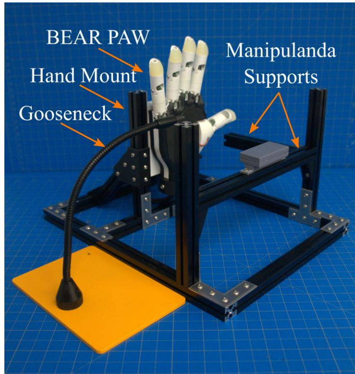
Figure 4-1. Depicts the testing platform for the BEAR PAW. It illustrates the hand mount used to hold the BEAR PAW stable during testing, the gooseneck which strategically held manipulanda, and the MakerBeam platform which supported the manipulandum used for individual digit articulation.
