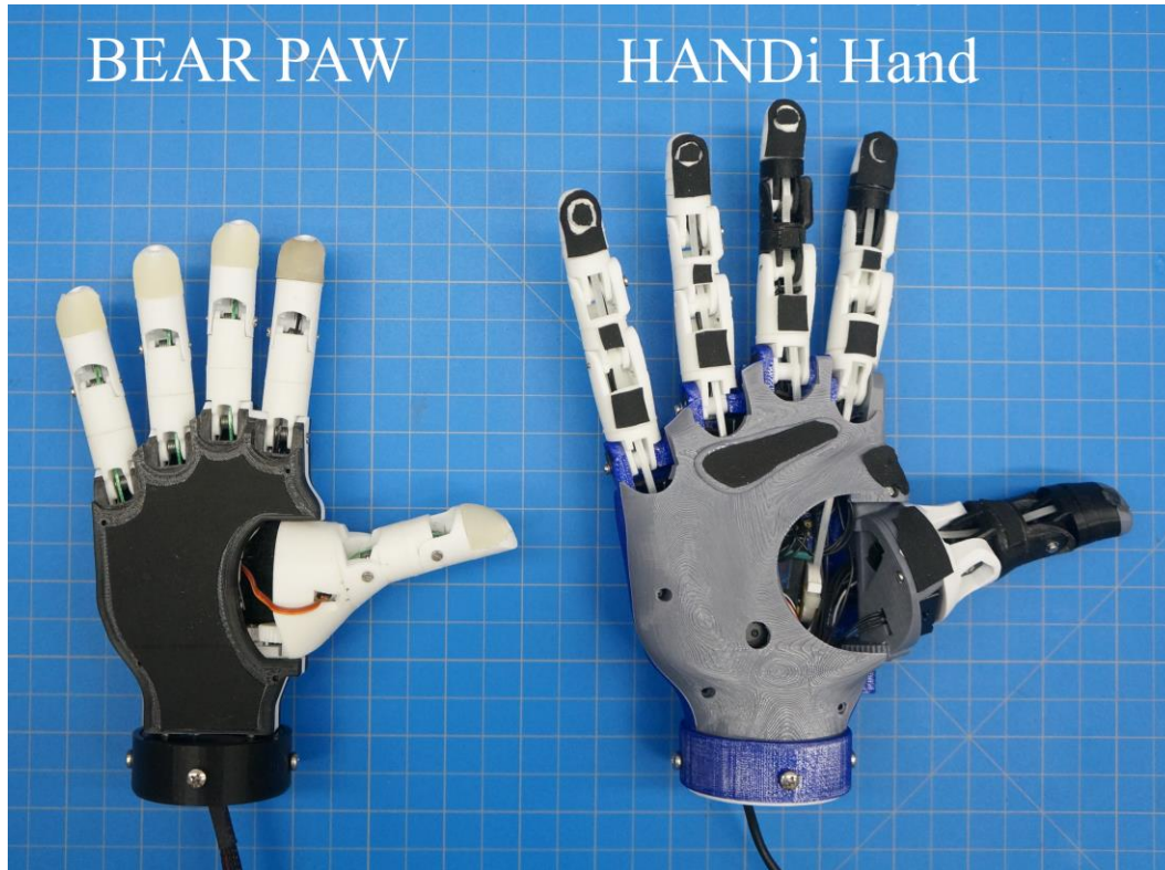
Figure 4-5. A size comparison between the BEAR PAW (left), a pediatric prosthetic hand, and the HANDi Hand (right), an adult prosthetic hand. Each square in the background is 1cm by 1cm.
