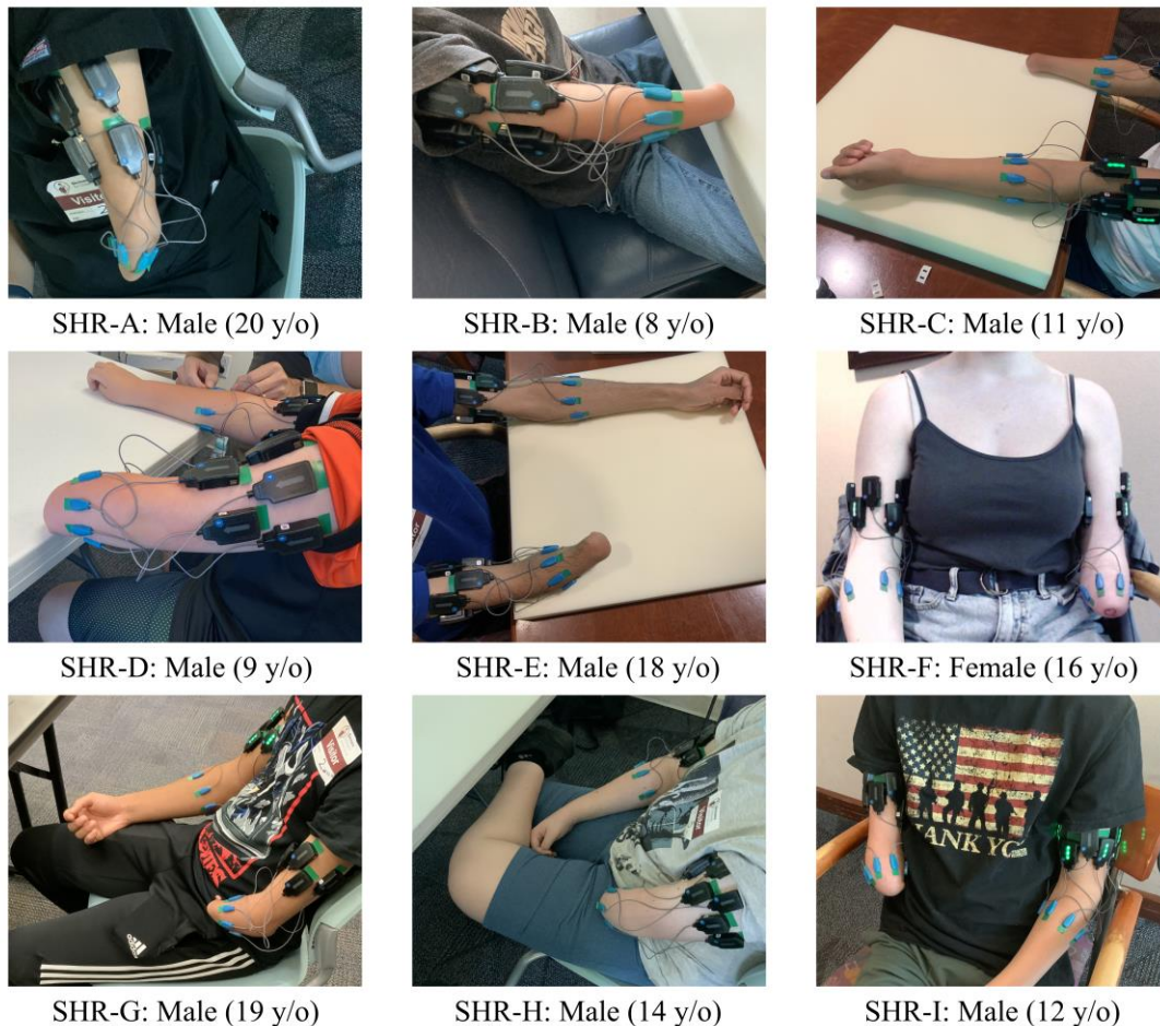
Figure 5-1. Participants with sEMG electrodes donned across unaffected and affected limbs with sex and age in years old (y/o) specified.
