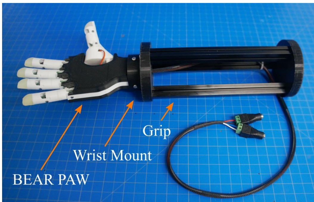
Figure 4-3. Depicts the testing rig used to perform the Anthropomorphic Hand Assessment Protocol, highlighting the BEAR PAW, wrist adapter mount, and forearm frame grip.
