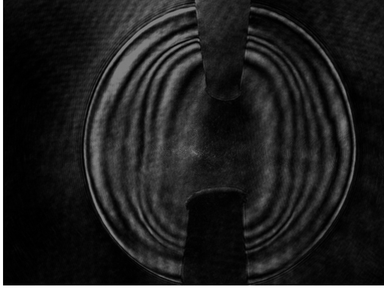
Figure G.10: Shadowgraph of shock front from 10 bar xenon discharge. The image is taken with a 3 ns YAG pulse timed 100s of nanoseconds after the discharge is initiated.
